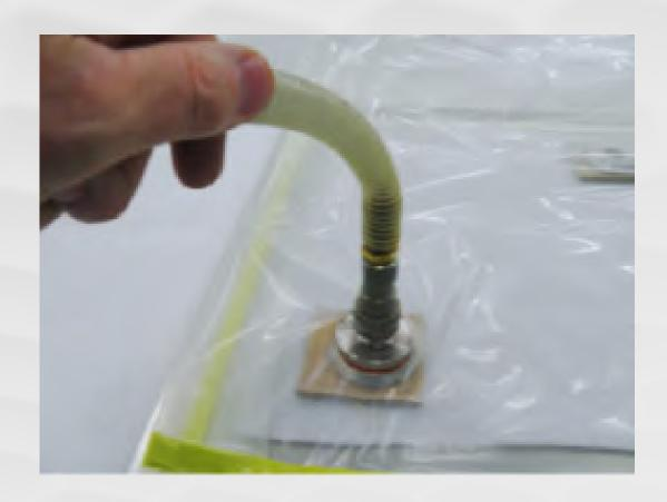
Mechanics have to fixate the vacuum hose in the correct position until full vacuum is reached. This may take up to 30 minutes when processing large parts for each vacuum valve.
