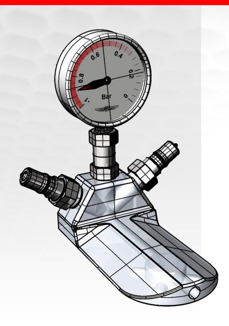
The SmartValve is invented by Bert Groenewoud. It solves the standard valve's tilting problems in the autoclave, oven and vacuum tables. Production files such as design drawings, STP / IGES files for 3D milling are created, making the SmartValve ready for production.
